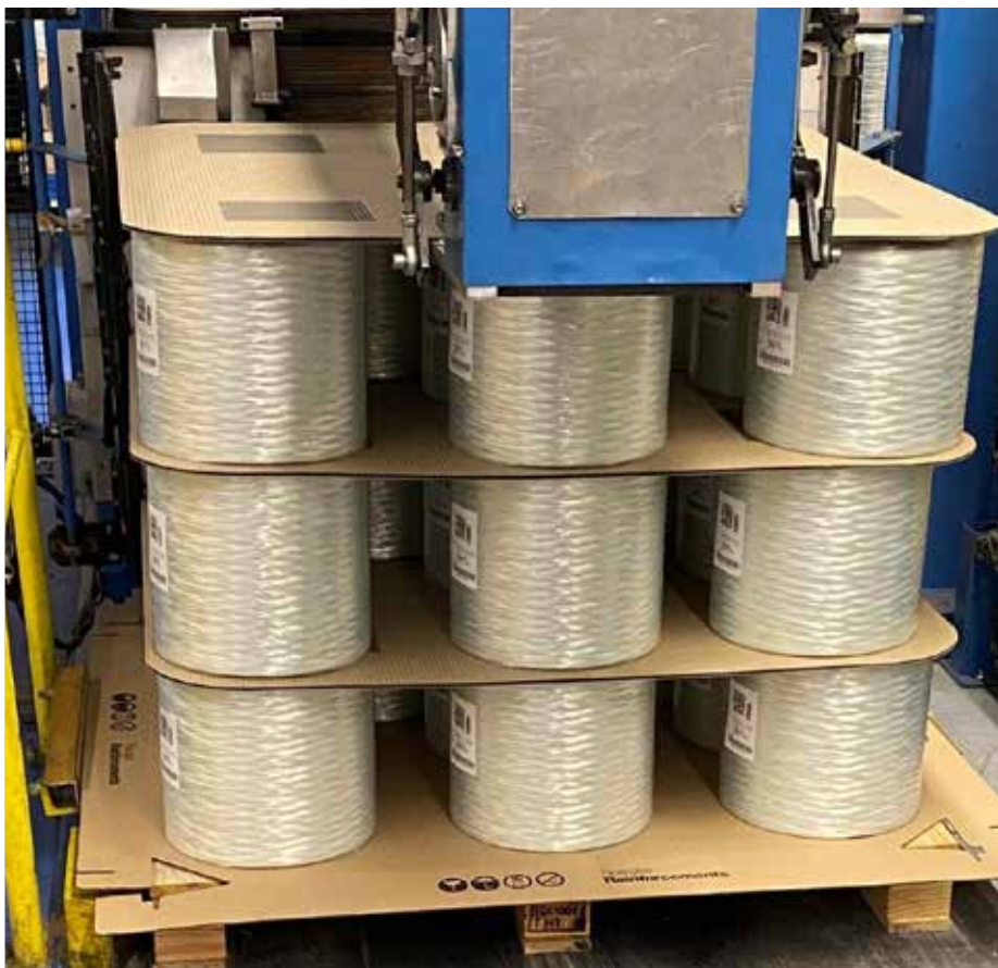
Photo submitted by: Valentin Richard | l'Ardoise, France Removal of the foam cardboard layers increased safety for the operator and provided an opportunity for a more sustainable solution for our customers.
